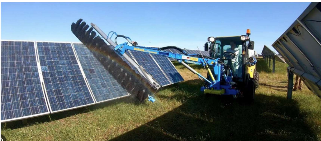
Photo 28 27 : Cleaning of Solar Arrays
